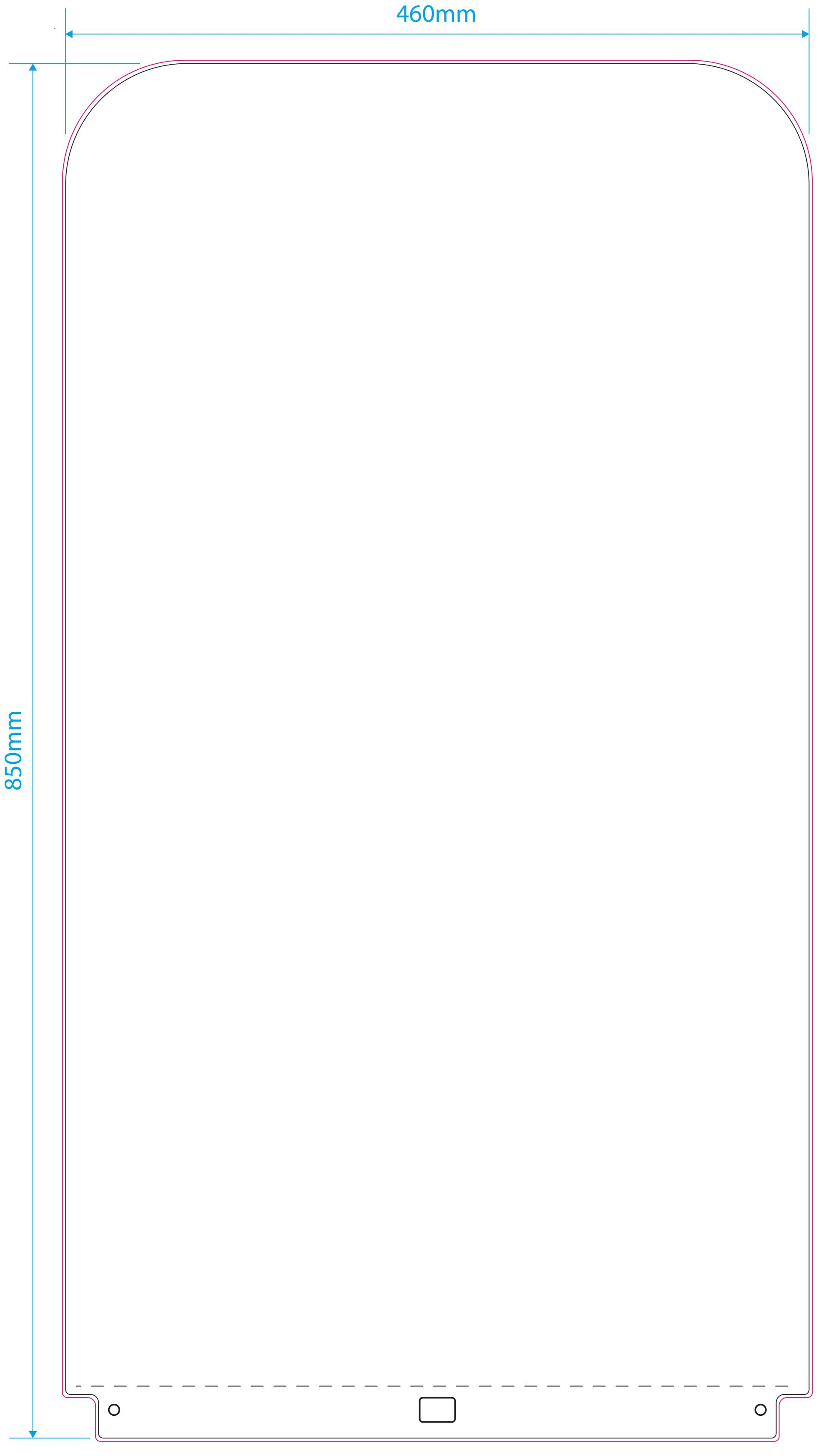
PLEASE NOTE: THIS AREA UNDERNEATH THE DASHED LINE IS NOT VISIBLE WHEN PANEL SLOTS INTO BASE.
